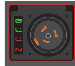
Line 2 and Neutral Reversed L2 and N - Red G, L1 - Green Border - Flashing Red
