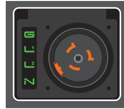
Correct G, L1, L2, N - Green Border - Solid White
