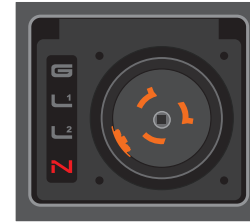
Missing Neutral N - Red G, L1, L2 - Off Border - Off
