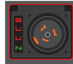
L1/L2 and Ground Reversed G, L1, L2 - Red N - Green Border - Flashing Red
