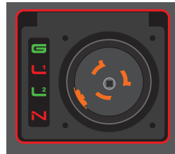
Line 1 and Neutral Reversed L1 and N - Red G, L2 - Green Border - Flashing Red
